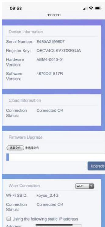
\*WiFi module must be configured before using the platform, and this operation is not required for 4G module.
