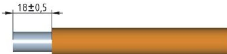
Step 3: put the protective wire sleeve into the cable.
