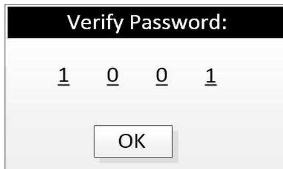
3) In the above interface, after entering the password, press the "ENTER" key to enter the following menu. The interface will display the current working mode. Press the "ENTER" key to select the required working mode through the "UP" and "DOWN" keys. Press the "ENTER" key again to confirm the selected mode, move the cursor to "OK", and press the "ENTER" key to confirm the input.
