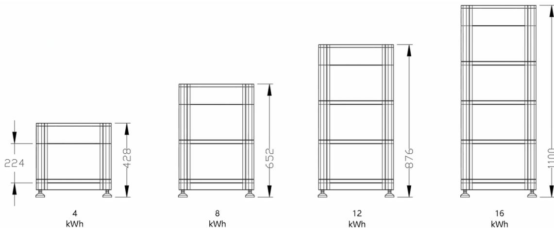
As shown in the figure above, the upper limit of the system stack is 20kwh, that is, 5 battery packs are stacked, the figure shows the size of the commonly used 1~4 battery pack stacking system, the connection between the battery packs is connected in series, please pay attention to whether the system voltage after series is in line with the load voltage range.
