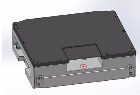
The batteries are installed by plug-ins, as shown in the figure on the right, which is the ground interface of each battery. When the batteries are installed by plug-ins, the ground wire will be directly connected without additional connection. Finally, all the ground wires will be exported through the ground interface of the main control module and connected with the ground port of the inverter (The battery interface of the main control module is shown in the left picture).
