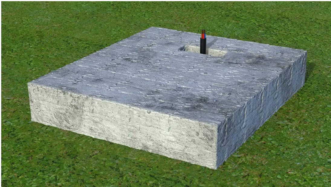
Fig. 3-1 Cabinet equipment cement foundation form 1 (KYT25kW-60kWh-A for example)
