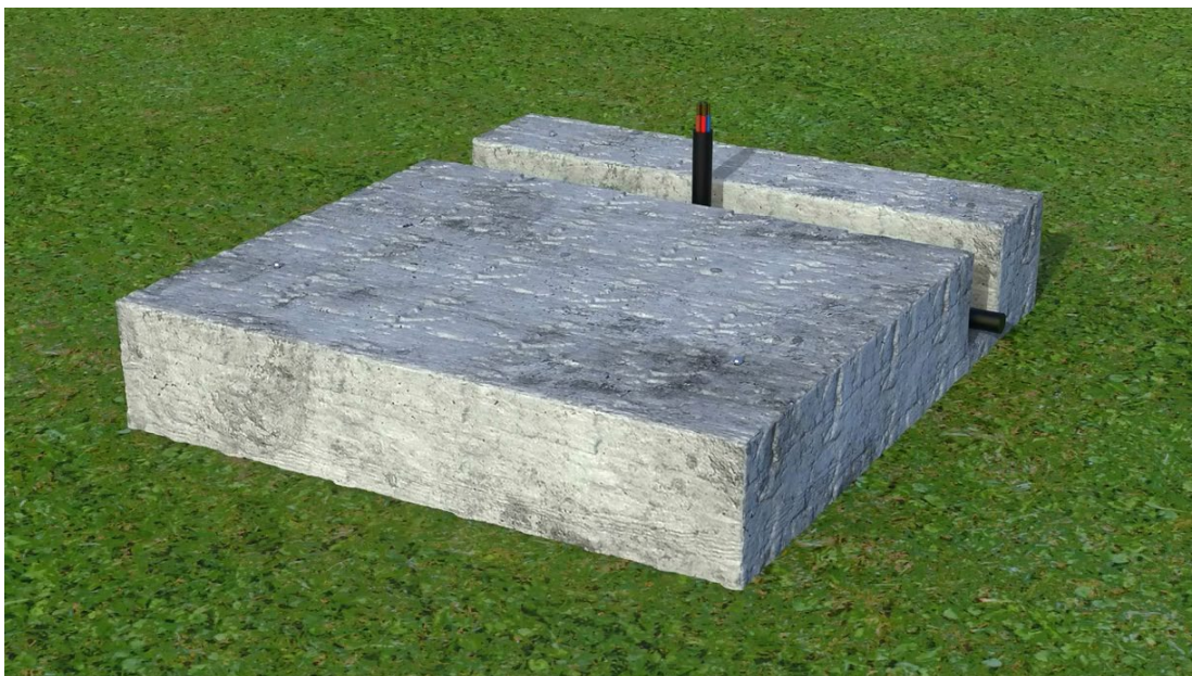
Fig. 3-2 Cabinet equipment cement foundation form 2 (KYT25kW-60kWh-A for example)
