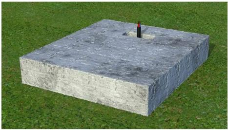
Fig. 5-3 Cabinet equipment cement foundation form 1
