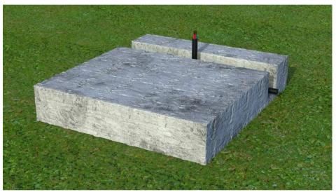
Fig. 5-4 Cabinet equipment cement foundation form 2
