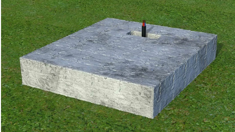
Fig. 5-3 Cabinet equipment cement foundation form
