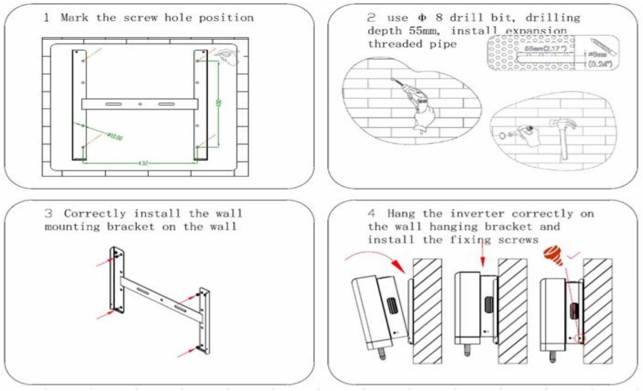
Step1: Mark the screw hole position;
