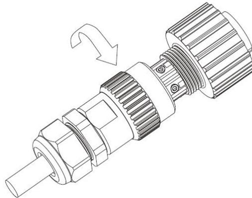
**Step 5:** Insert the socket into the AC output terminal, screw the socket clockwise, and loosen the socket anticlockwise.
