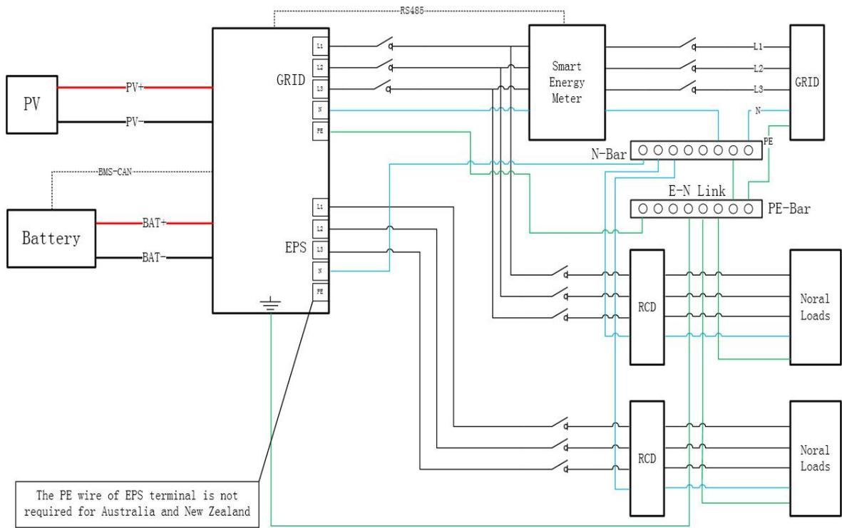
Neutral line of alternative supply must be disconnected after the grid is off (applies to other counties).
