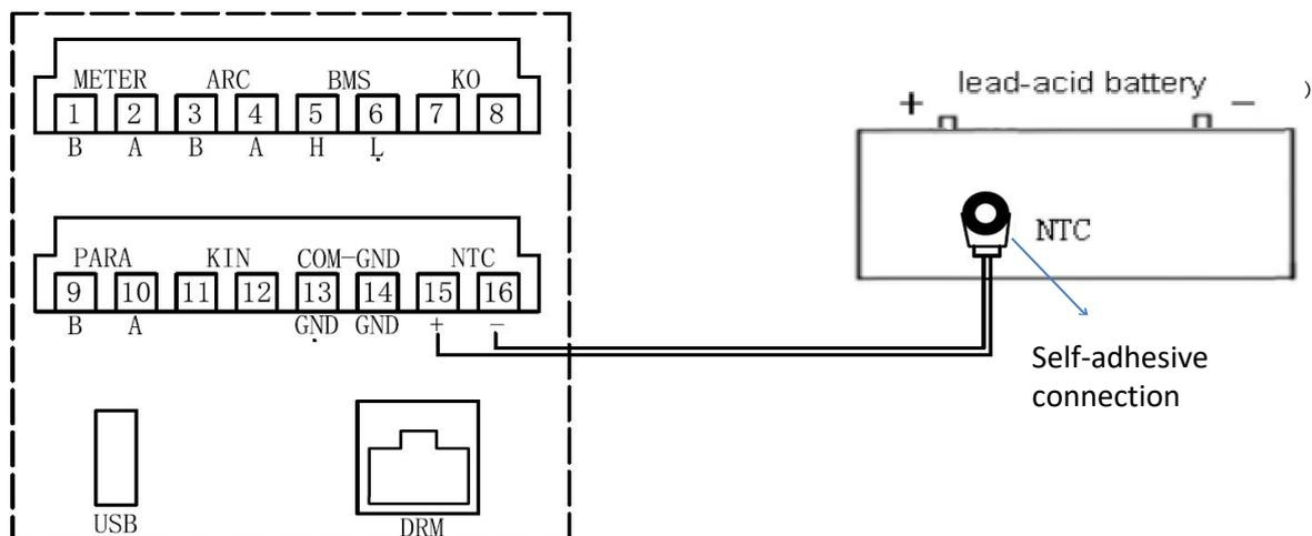
The inverter adjusts the output power when it detects the temperature of NTC, as shown in the following table:
