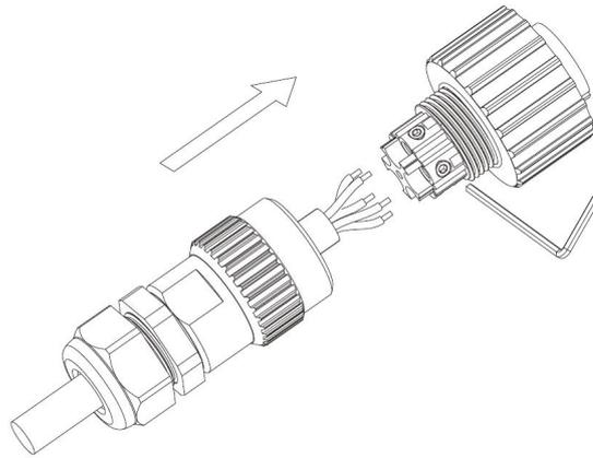
Figure loosening connector screws(the GRID terminal is black)
