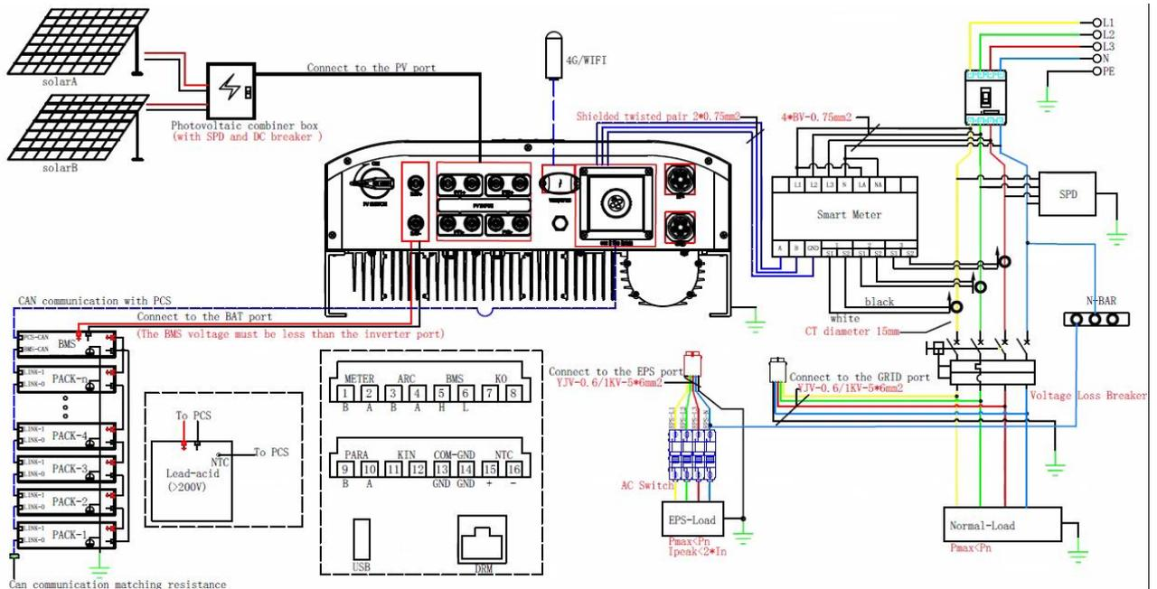
If the user requires that the load of EPS cannot be powered off, a dual power switch needs to be added, please connect it as shown in the figure below:
