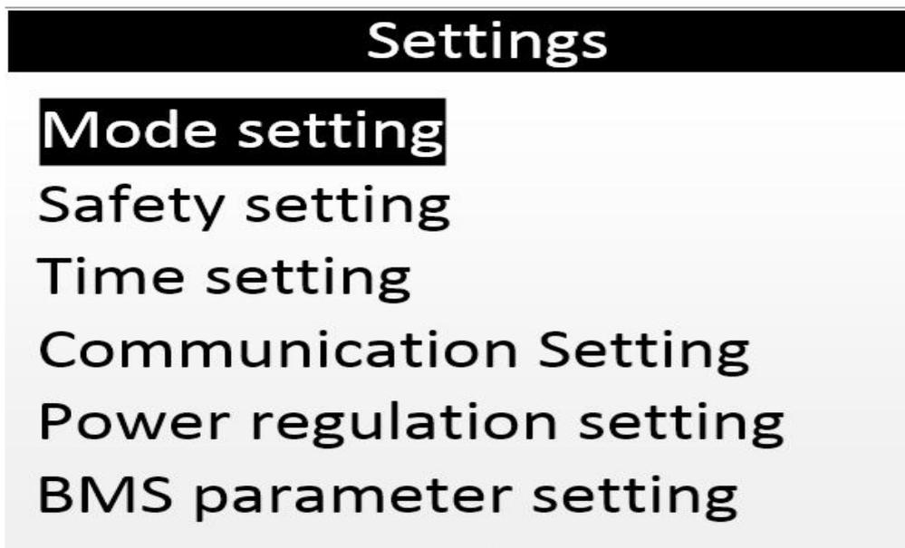
3) Press the "ENTER" button in the above interface to enter the password interface, as shown in the following menu. The default password is "1001". Press the "ENTER" button to select the cursor and add or subtract the value through the "UP" and "DOWN" buttons, then press the "ENTER" button again to confirm the value at the optical mark, then move the cursor to "OK", and press "ENTER" to confirm the input.
