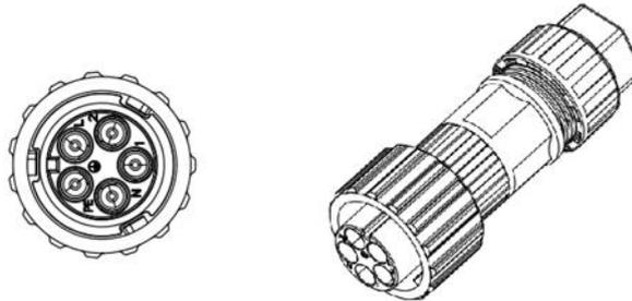
b) Protective earthing (second PE at external enclosure)
