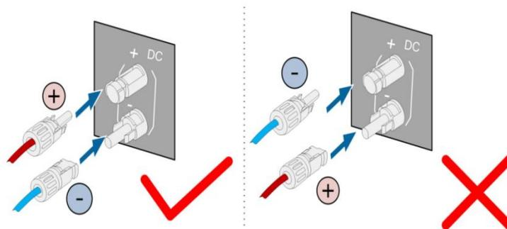
2). Arc or contactor over-temperature may occur if the PV connectors are not firmly in place, and KOYOE shall not be held liable for any damage caused due to this operation.
