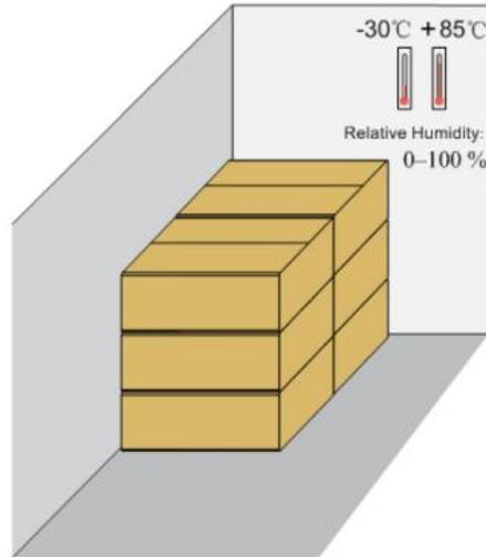
Fig. 6-3 Example of Inverter Storage
