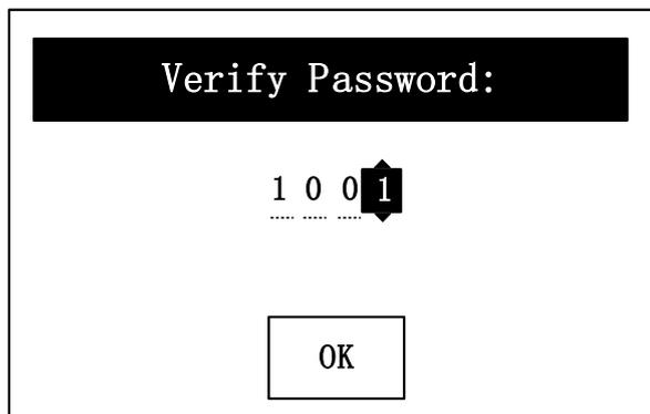
4) Under the above interface, after entering the password, press the "ENTER" key to enter the following menu, the interface will display the current working mode, press the "ENTER" key, select the desired working mode through the "UP", "DOWN" button, press the "ENTER" button again to confirm the selected mode, move the cursor to "OK", press the "ENTER" key and confirm the input.
